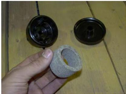
**Clean** the filter using compressed air, blow the filter from the inside out. Holding the filter up to a light, inspect the filter. If there is any light visible through the filter, discard the filter and cartridge and replace with a new one
