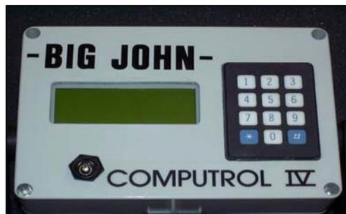
In the "OFF" position, the toggle switch on the Big John remote screen will stop or prevent the seed shaft, dividers/single drops, slides, and alley wipers from moving.
