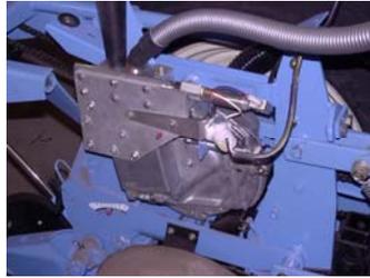
**Remove the cover** from the planter. Inspect the cover for any obvious problems, such as broken or missing parts. Move the slide back and forth to make sure it glides freely in its tracks. The slide should operate on as little as 10 PSI. If it does not, the slide will have to be disassembled and cleaned.
