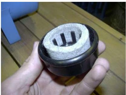
**Place** the filter element into the base. Look to make sure that it is not pushed down far enough into the base that with the lid on there is room for unfiltered air to move around the filter and into the compressor. Place the lid on the cartridge.
