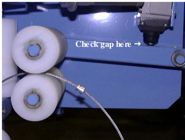
**For proper adjustment:** Place the cable inside the checkhead rollers as shown. Loosen the two adjustment screws on the limit switch and adjust it so that the limit switch button comes in slight contact with the trip (see arrow).
