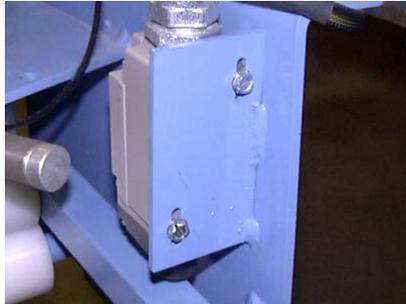
**To adjust the checkhead** for different cable sizes, there are two adjustment screws which allow the limit switch to move up or down.
