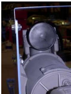
**Reinstall** the cartridge without using any sealing agent on the threads. This will prevent anything from coming off of the threads and into the compressor. The plastic will seal by itself.
