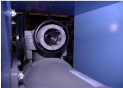
**Remove** the filter element from the cartridge by first unsnapping the lid. Take the filter out of the cartridge, being carefully not to tear it. You may remove the entire cartridge by unthreading it from the compressor head to make it easier to service.
