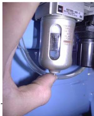
**To drain the water out of the accumulator**, press up on the drain valve located on the bottom of the accumulator. Some models may be equipped with a turn valve for the drain. Note: this is the reservoir located on
